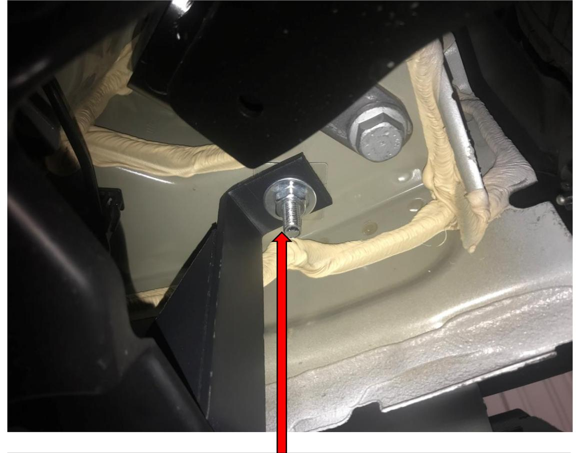
Remove the sticky cover on the chassis at the rear of the vehicle this just peels off to reveal a large hole place the large T-bolt into the hole and then tighten.
