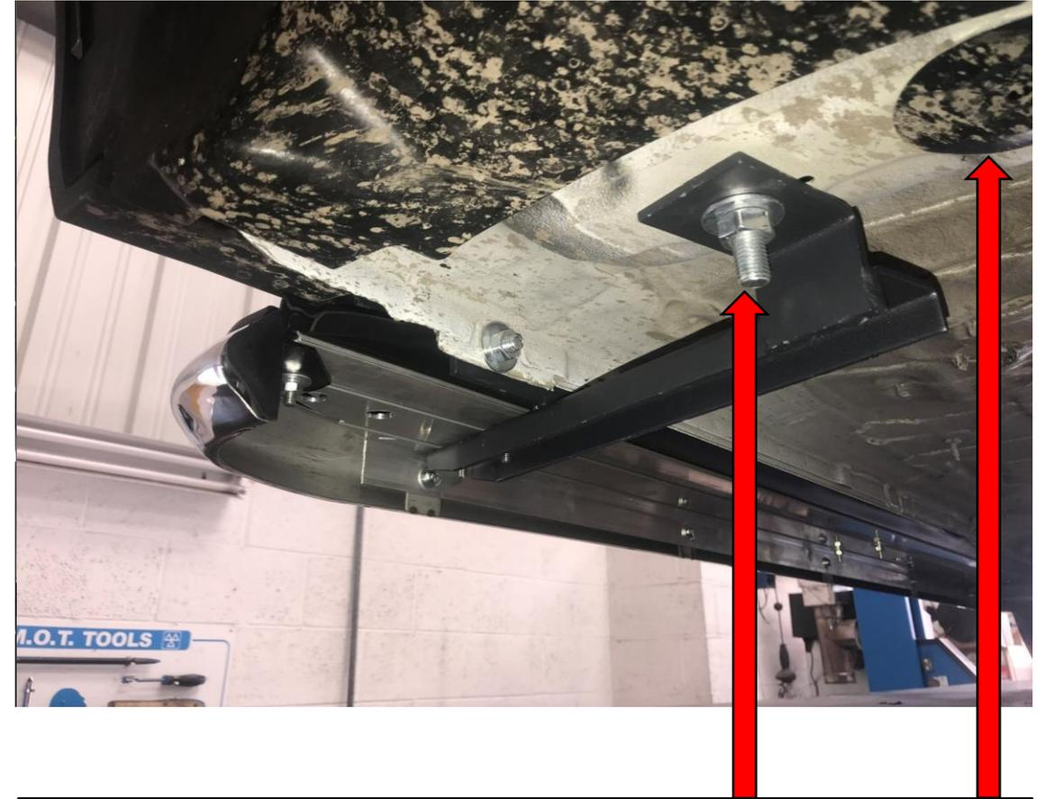
For the front bracket first remove the grommet nearest to the sill (this is a large plastic fitting that unscrews to leave a hole in the chassis). There are two grommets that are located on each side close to the front of the vehicle then use the large T-bolt to slot into the hole and tighten.
